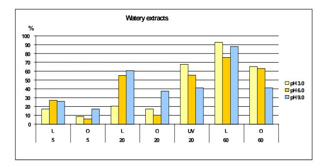
*Figure 3.* Color losses of watery and ethanolic extracts after 21 days of storage, expressed like % absolute absorbance losses at 430 nm. L -solar light, O-darkness, UV- UV light, the practiced temperatures 5°C, 20°C and 60°C
