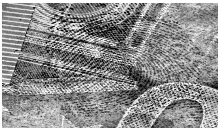
Fig.3 – Fingerprint rendered with indandione on a 50 EURO paper banknote, viewed with a RUVIS UIS-ImaQuest device (Universal Imaging System).
