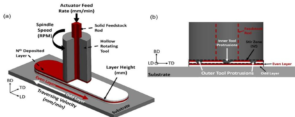
**Fig. 2.** a) Schematic of AFSD process parameters, illustrating the essential elements and variable parameters; b) Schematic of feature tool protrusions in interaction with layers that have already been deposited [2]
