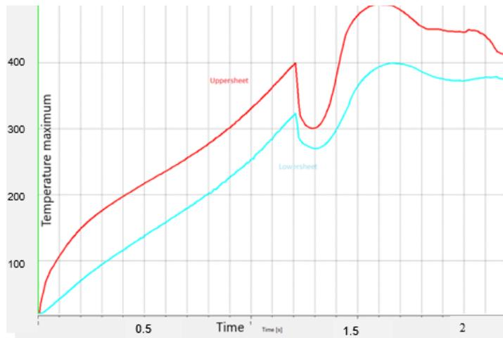
**Fig. 10.** Maximum temperature for the upper sheet and the lower sheet during the process (the Time [s] and Temperature maximum [°C])
