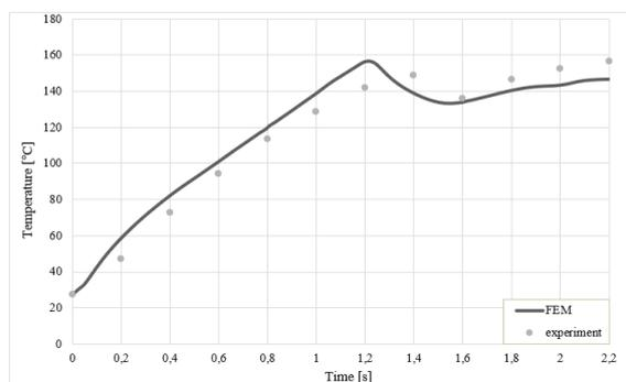
**Fig. 19.** Variation in temperature throughout the welding process at the specified measuring point, Sensor 2 [15]
