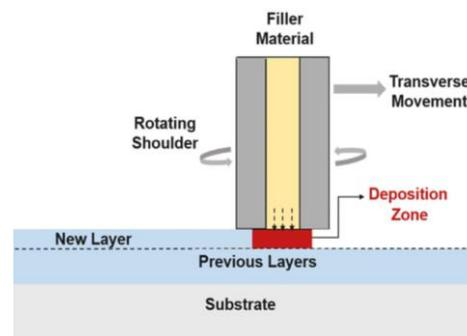
**Fig. 1.** Schematic of additive friction stir deposition (AFSD) [1]
