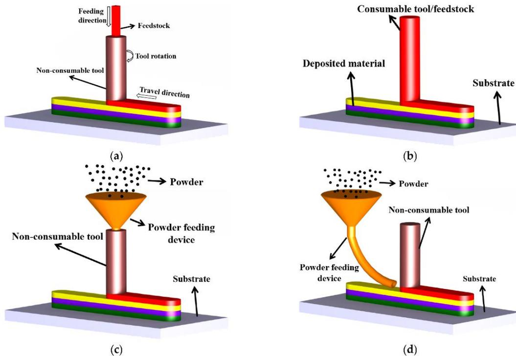
**Fig. 3.** Schematic of the AFSD process with different modes: a) rod with non-consumable tool; b) consumable tool; c) powder with non-consumable tool; d) powder with non-consumable tool [3]
