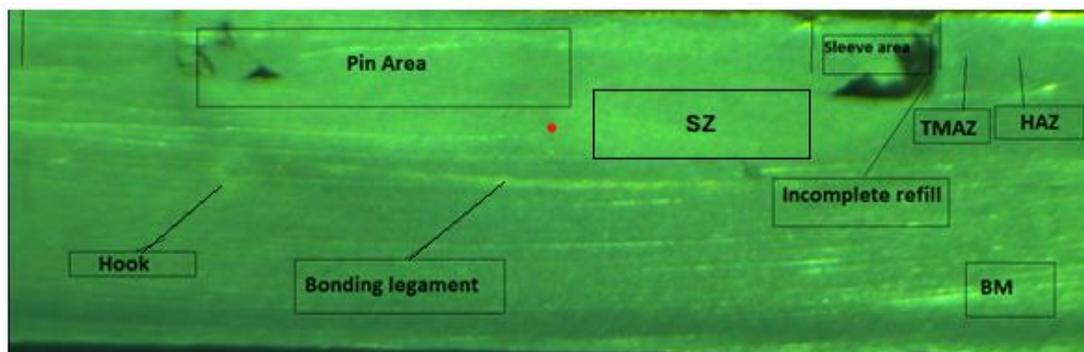
Fig. 20. Cross-section through the welded joint
