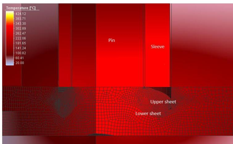
**Fig. 11.** Temperature field during FSW with filler material
