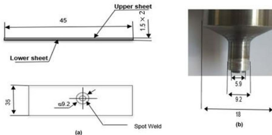
**Fig. 4.** Welding equipment: (a) sheet metal dimensions, (b) FSW tool dimensions
