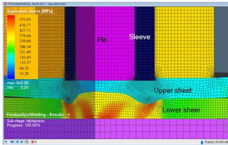
**Fig. 7.** Von Mises equivalent stress during FSW without filler material
