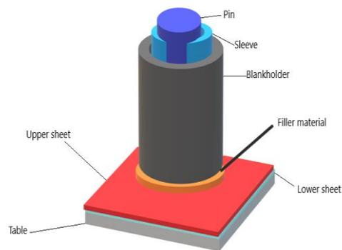
**Fig. 5.** The model used in the numerical modelling
