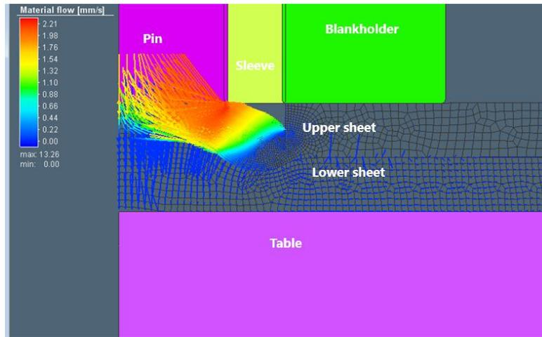
**Fig. 12.** Material flow during FSW with filler material
