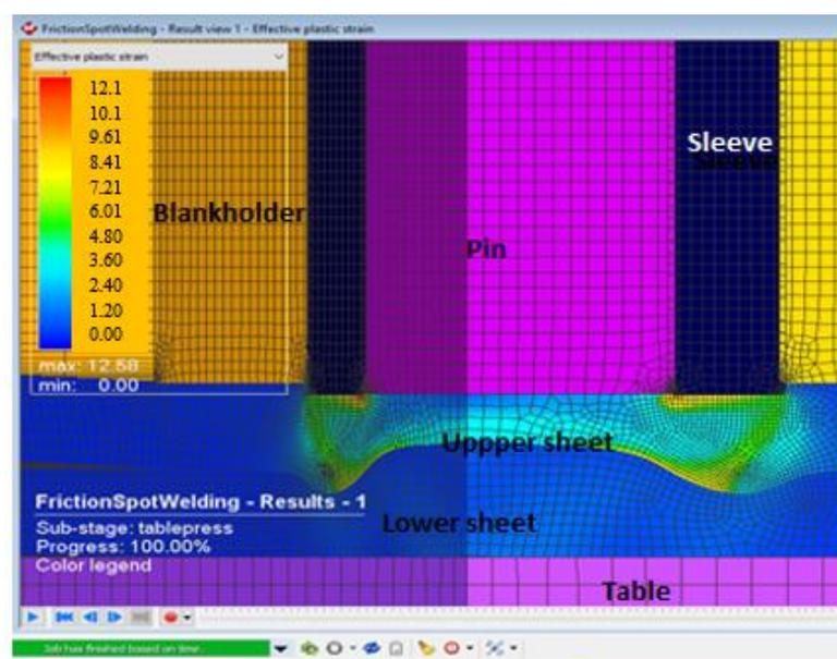
Fig. 6. Effective plastic strain during FSW without filler material
