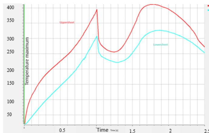
**Fig. 14.** Maximum temperature for the upper sheet and the lower sheet during the process (Time [s] and Temperature maximum [°C])
