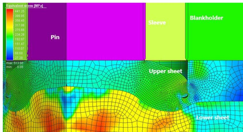
**Fig. 13.** Equivalent stress during FSW with filler material
