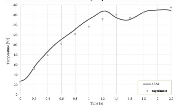
**Fig. 18.** Variation in temperature throughout the welding process at the specified measuring point, Sensor 1 [15]
