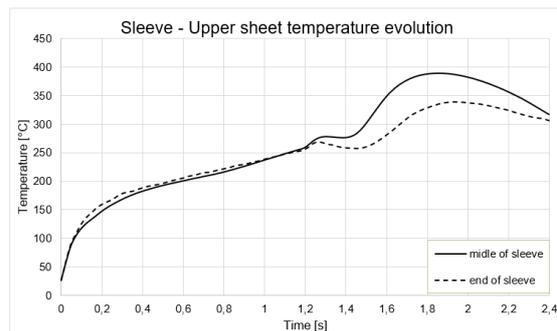
**Fig. 17.** Temperature at sleeve-upper sheet interface – FEM [15]
