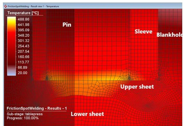
**Fig. 9.** Temperature field during FSW without filler material
