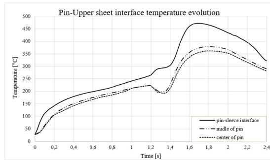
**Fig. 16.** Temperature at pin-upper sheet interface – FEM [15]
