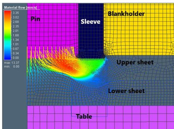
**Fig. 8.** Material flow during FSW without filler material
