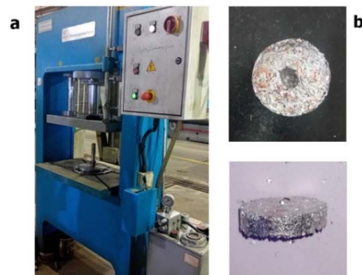
Fig. 3. Chips pre-compact: a) compaction machine; b) compacted chips
