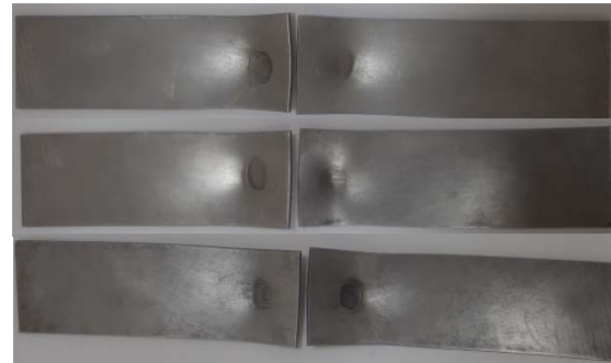
Fig. 16. Broken specimens after the tensile test for different applied pressures: P13 at the top, P14 in the middle and P15 at the bottom
