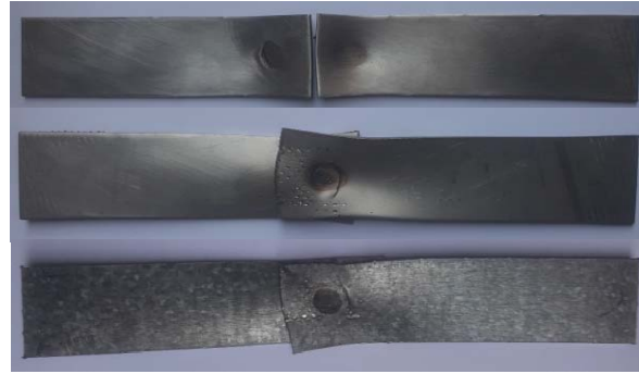
Fig. 5. Broken specimens after the tensile test for different materials: P1 at the top, P2 in the middle and P3 at the bottom
