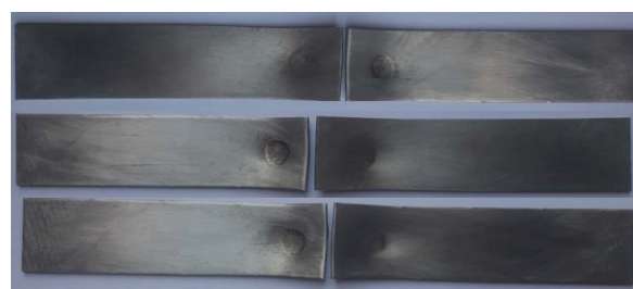
Fig. 8. Broken specimens after the tensile test for different welding times: P4 at the top, P5 in the middle and P6 at the bottom
