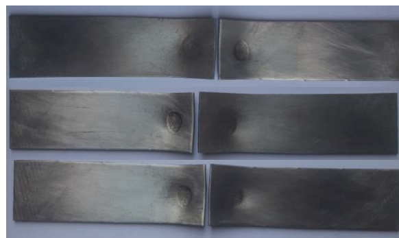
Fig. 11. Broken specimens after the tensile test for different current intensities: P7 at the top, P8 in the middle and P9 at the bottom
