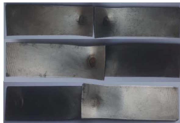
Fig. 14. Broken specimens after the tensile test for different sheet thickness: P10 at the top, P11 in the middle and P12 at the bottom
