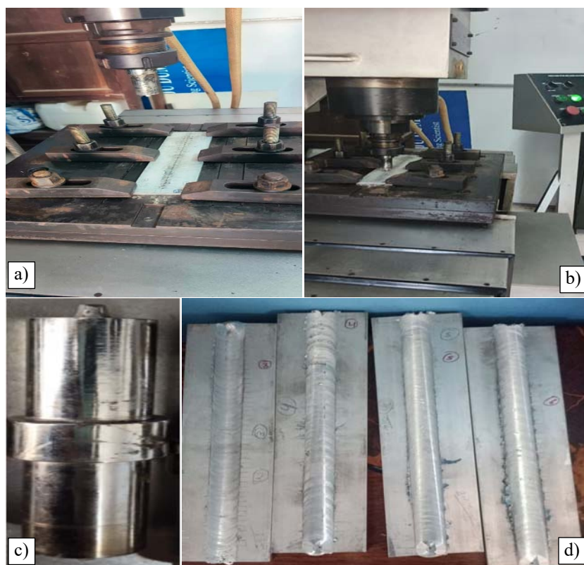
Fig. 2. FSP processing of AA6061: a) AA6061 plates before FSP process; b) AA6061 plates during FSP process; c) FSP tool; d) AA6061 samples reinforced with SiC and CuO by FSP method
