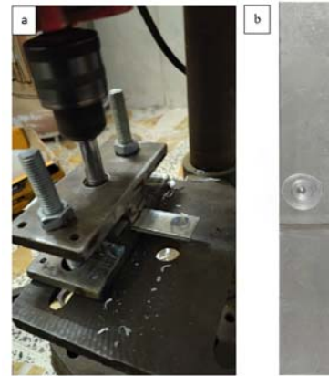
Fig. 1. Joining process: a) fixtures of the specimen; b) the specimen
