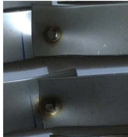
Fig. 3. Specimens after the tensile-shear test
