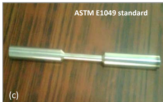
Fig. 1. Equipment and materials: a) high-speed CNC lathe; b) fatigue testing setup; c) fatigue test specimen
