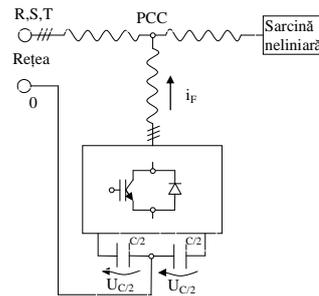
Fig.9. Shunt active power filter with 4 wires and median point on capacity
