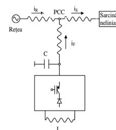
Fig.4. Shunt active power filter current source inverter
