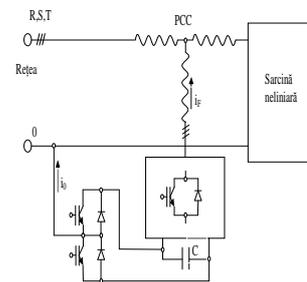
Fig.10. Shunt active power filter with 4-wire and 4-pole
