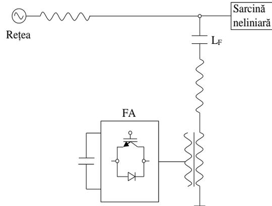
Fig.13. Active power filter in series with shunt passive filter
