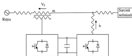
Fig.7. Hybrid active power filter, UPFC
