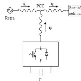
Fig.3. Shunt active power filter with voltage source inverter
