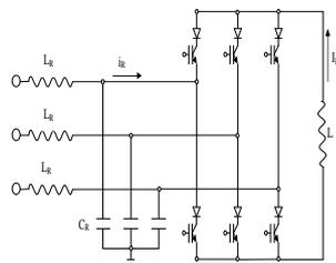
Fig.2. Three-phase current inverter
