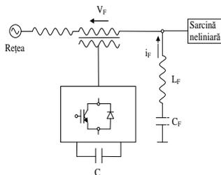
Fig.8. Hybrid filter, active series and shunt passive
