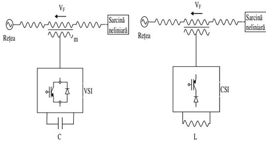
Fig.5. Series FAP - voltage source inverter
