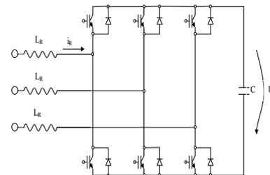
Fig.1. Three phase voltage inverter
