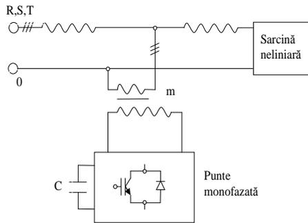
Fig.11. Active power filter series with 3 single-phase inverters
