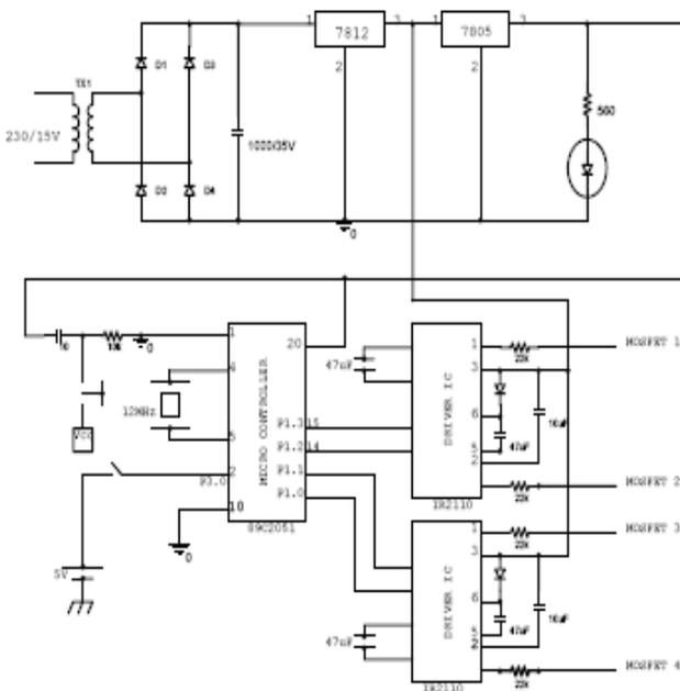
Fig. 11. Control circuit for generating the Driving Pulses.
