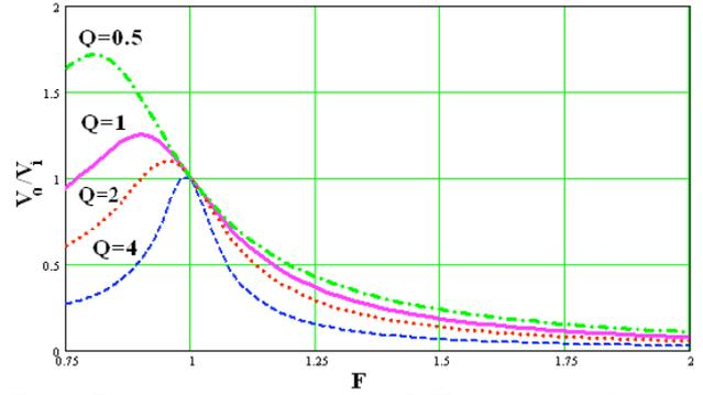
Fig.4. Frequency response of the LCL resonant tank
