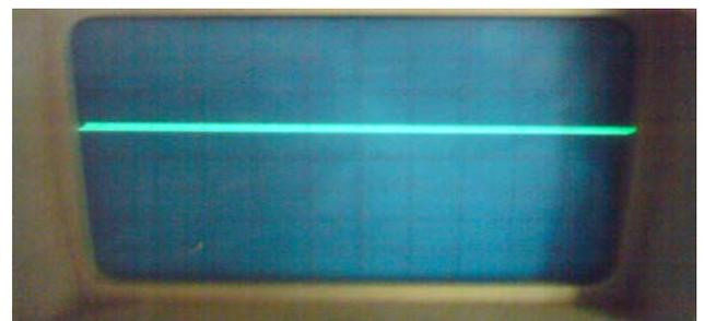
(e) Output of DC-DC Converter. (Load Voltage)
