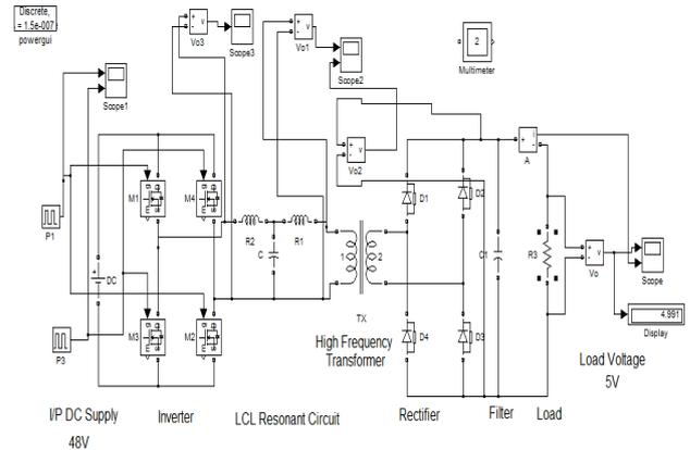
Fig. 5. LCL Resonant DC-DC Converter
