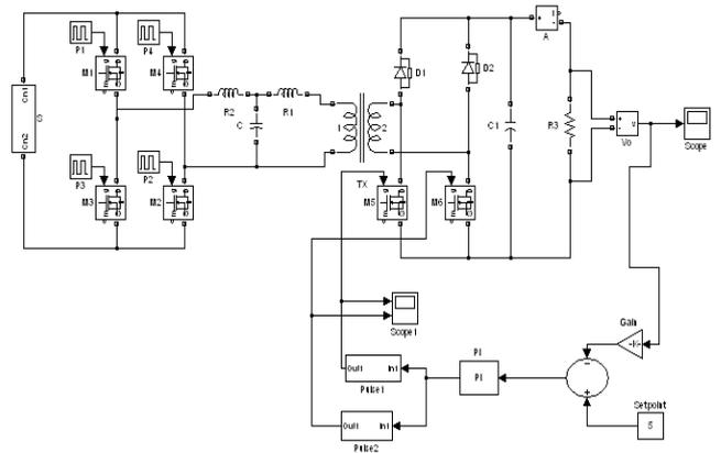
Fig. 7. Closed loop controlled LCL Resonant DC-DC Converter
