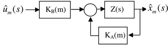
Fig.2. Feedback schematic for the spatial mode m
