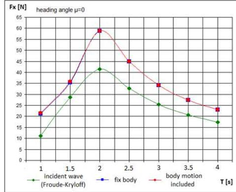
Fig. 5. Surge diffraction forces, heading angle  $\mu = 0^\circ$
