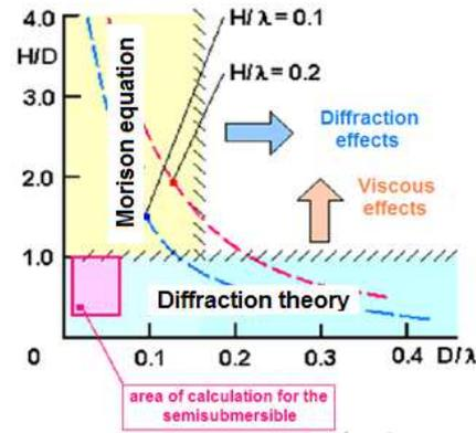
**Fig. 2.** Definition of calculation area for the SR 192 semisubmersible
