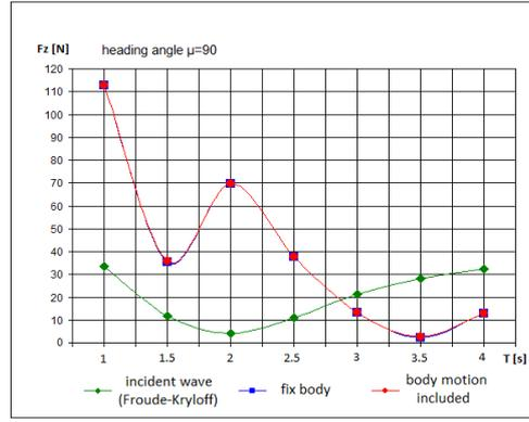
Fig. 11. Heave diffraction forces, heading angle  $\mu = 90^\circ$
