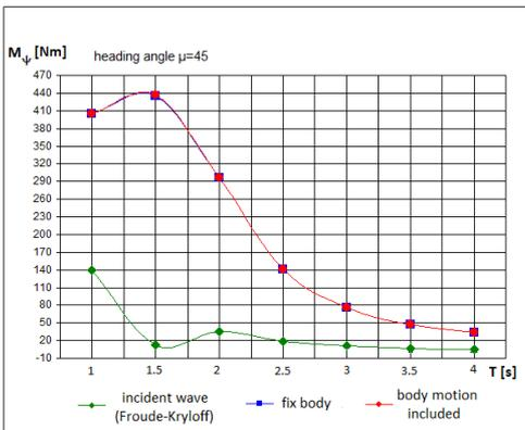
Fig. 16. Yaw diffraction moments, heading angle  $\mu = 45^\circ$
