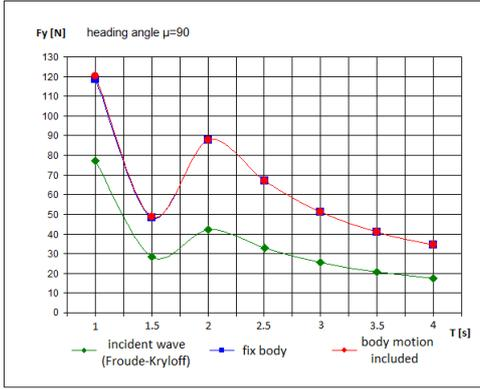
Fig. 8. Sway diffraction forces, heading angle  $\mu = 90^\circ$
