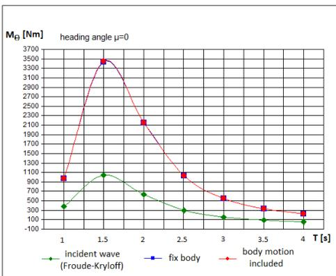
Fig. 15. Pitch diffraction moments, heading angle  $\mu = 0^\circ$
