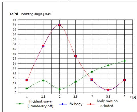
Fig. 10. Heave diffraction forces, heading angle  $\mu = 45^\circ$
