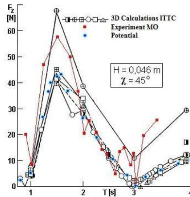
Fig. 17. Vertical diffraction forces  $F_z$ , comparative results, heading angle  $\mu = 45^\circ$
