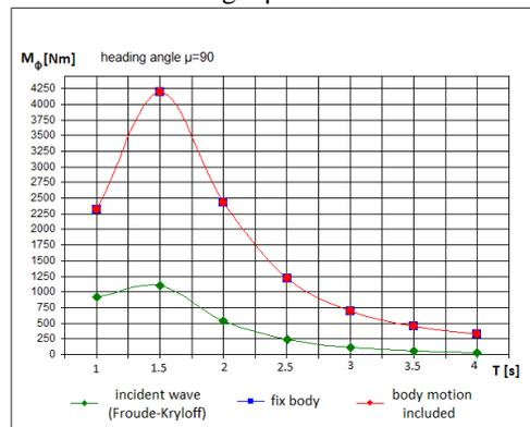
Fig. 13. Roll diffraction moments, heading angle  $\mu = 90^\circ$
