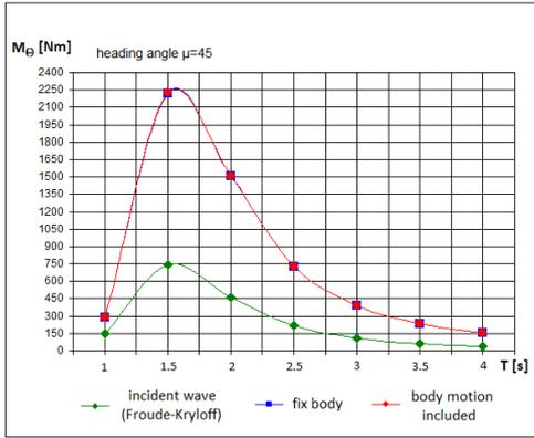
Fig. 14. Pitch diffraction moments, heading angle  $\mu = 45^\circ$
