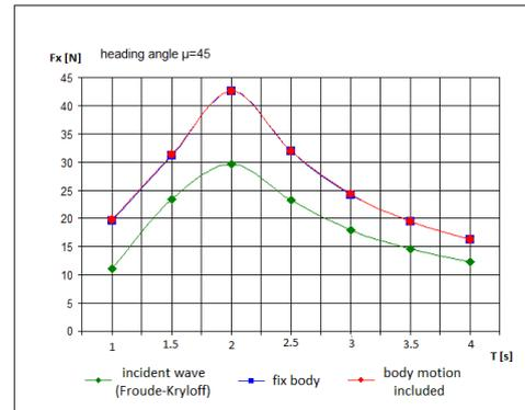
Fig. 6. Surge diffraction forces, heading angle  $\mu = 45^\circ$
