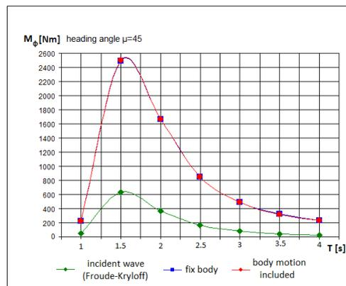
Fig. 12. Roll diffraction moments, heading angle  $\mu = 45^\circ$
