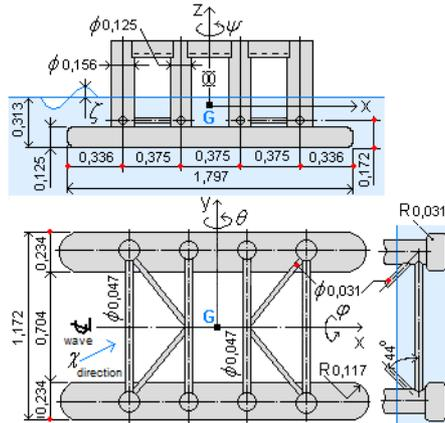
**Fig. 1.** The geometry of the semisubmersible model (scale 1:64)
