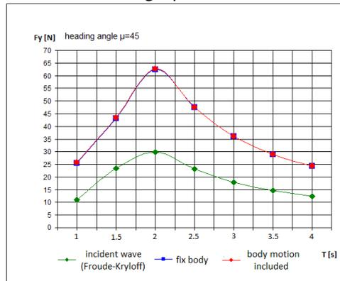
Fig. 7. Sway diffraction forces, heading angle  $\mu = 45^\circ$
