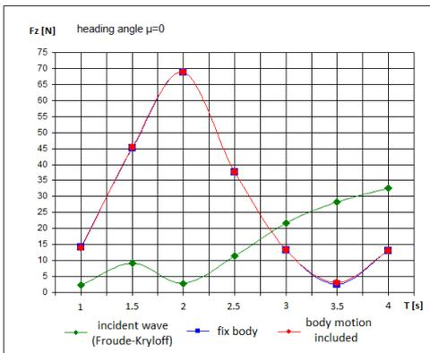
Fig. 9. Heave diffraction forces, heading angle  $\mu = 0^\circ$
