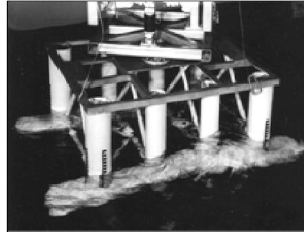
Photo 2. The semisubmersible model coupled to the six components dynamometer
