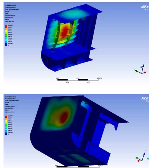
Fig. 10 Double bottom unit total deformation spots.
