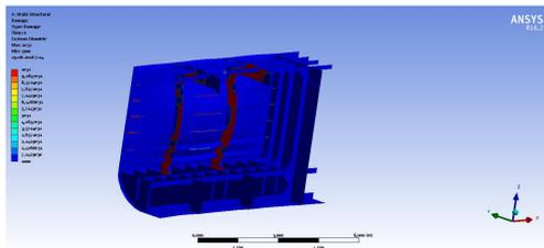
**Fig. 16.** Fatigue damage for the double bottom model
