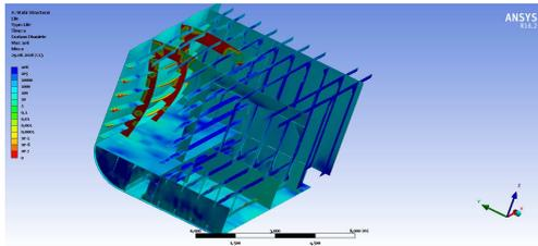
**Fig. 15.** Fatigue life for the double bottom model
