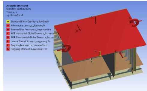
Fig.2 Pressure loads and moments that act to the double bottom unit
