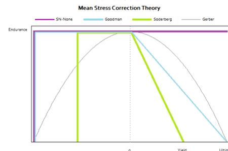
**Fig. 14** Graphical representation of the Goodman, Shoderberg, Gerber mean stress along with the S-N data.
