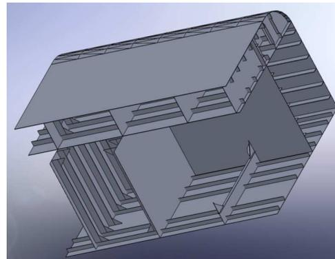
**Fig.1** SolidWorks 2015 double bottom model.
