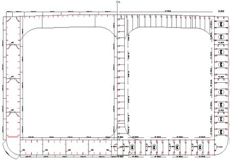
**Fig. 1a)** Cross-section area at the amidships section
