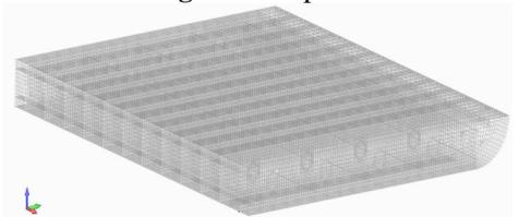
Fig. 7 Meshed double-bottom structure
