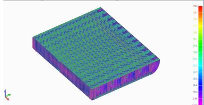
Fig. 12 Global stress ( VonMisses), in case of the bordering lack
