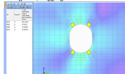
**Fig. 17b) Sagging - Bordered cut out**
