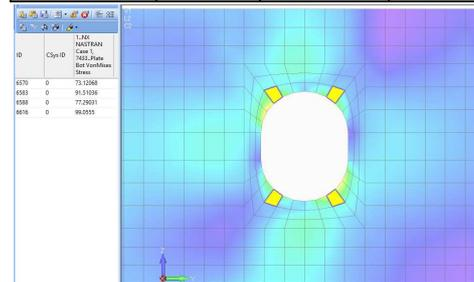
**Fig. 17a) Sagging - Unbordered cut out**
