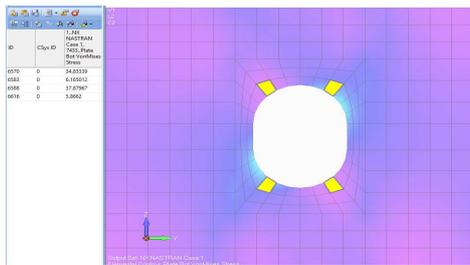
**Fig. 16a) Hogging - Unbordered cut out**
