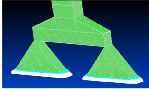
**Fig.6** Mesh detail and the external loads applied to the crane
