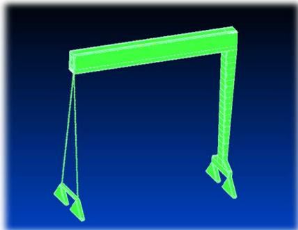
**Fig. 5** Discrete structure of the crane
