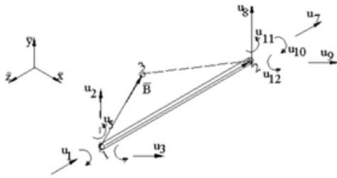
Fig. 1 Beam elements in space
