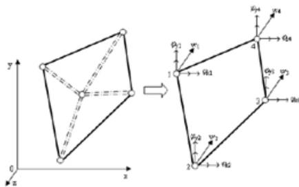
Fig. 3 Quadrilateral finite element
