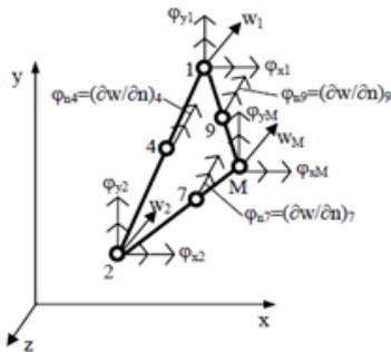
Fig. 2 Triangular finite element of shell type thin plate -release degree presentation
