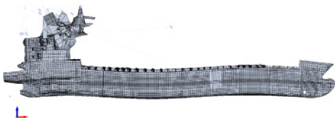
Fig. 16 FE model- Dry, Global vertical mode 3: 14.26 Hz
