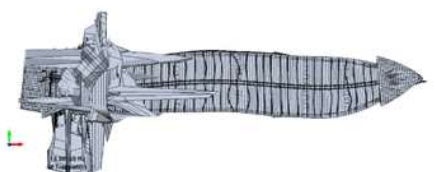
Fig. 19 FE model- Dry, Global horizontal mode 3: 18.86 Hz
