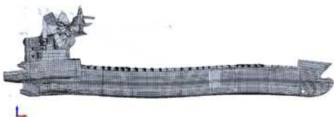
Fig. 16 FE model- Dry, Global vertical mode 3: 14.26 Hz
