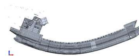
Fig. 14 FE model- Dry, Global vertical mode 1: 3.91 Hz
