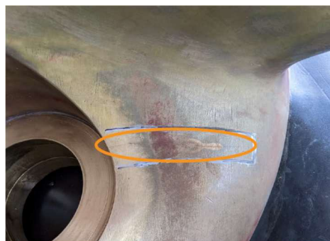
a) Surface cracks on blade no 2
