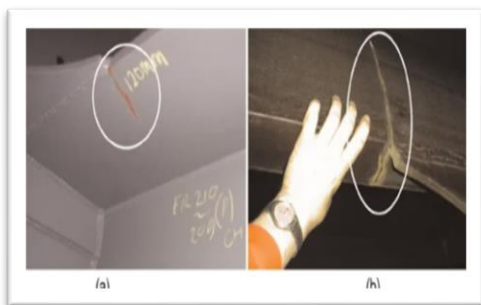
Fig.4 Cracks in ship structure caused by vibrations [6].
