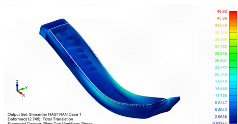
Fig.20 Ballast condition results: 2D elements – sagging
