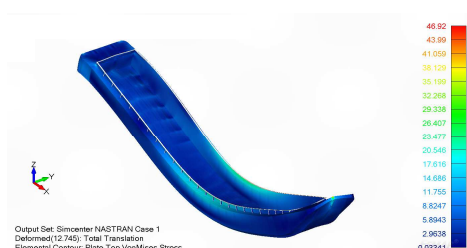
Fig.20 Ballast condition results: 2D elements – sagging
