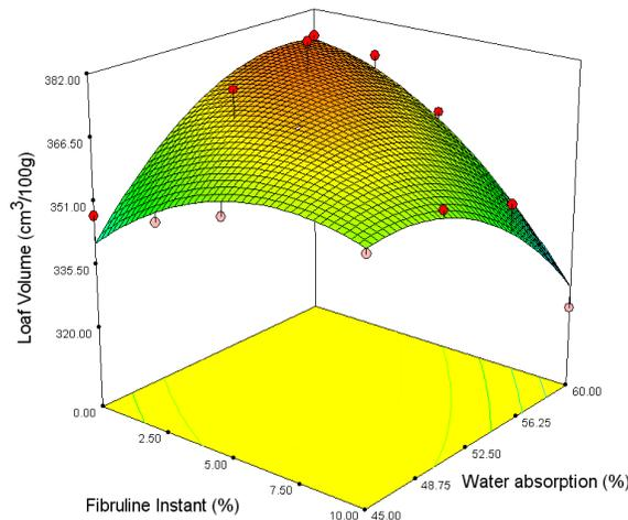
**Figure 1.** Response surface plot showing the combined effects of Fibruline Instant level and water absorption level of wheat flour on loaf volume of bread samples
