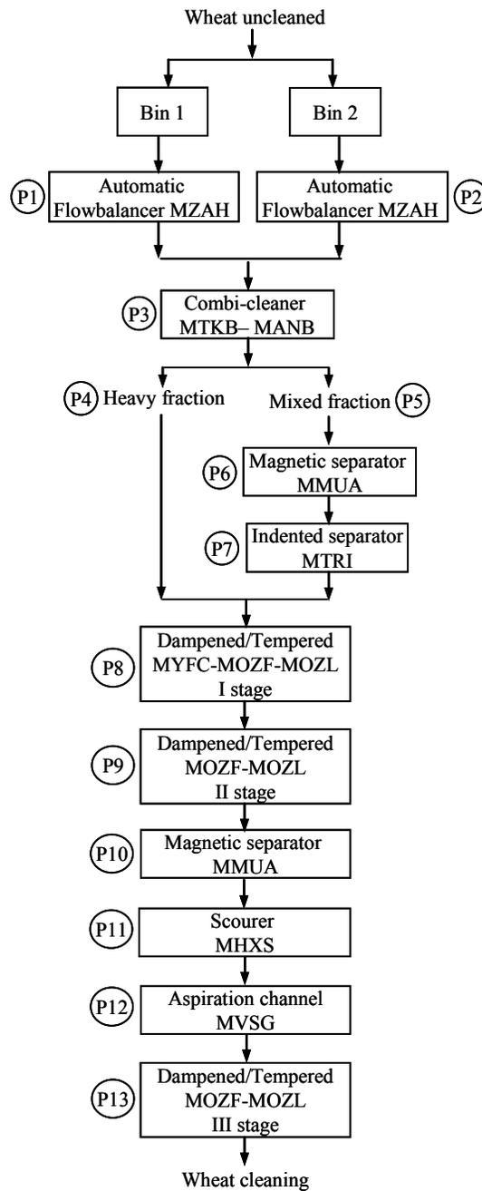
Figure 1. Technological diagram of the cleaning section
