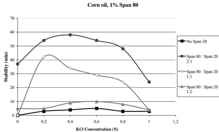
**Figure 5.** Stability of reverse double emulsions versus the concentrations of KCl, in relation with the ratio between the concentrations of Span 20 and Span 80
