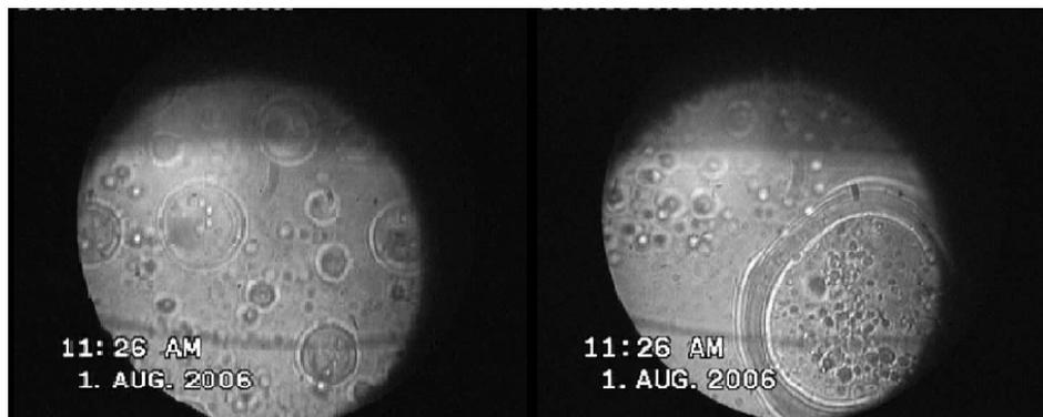
**Figure 3.** Appearance of the emulsion containing 25% (v) 1 N KCl solution and 75% (v) corn oil in the presence of 1% (m) Span 80: a) kinetics at the beginning of the reaction, b) after a few dozen seconds
