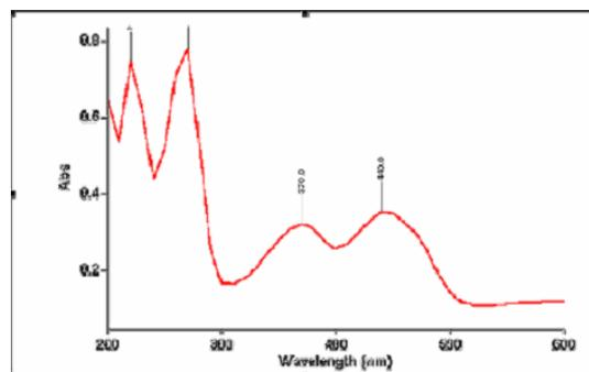
**Figure 2.** UV VIS standard spectre for riboflavin
