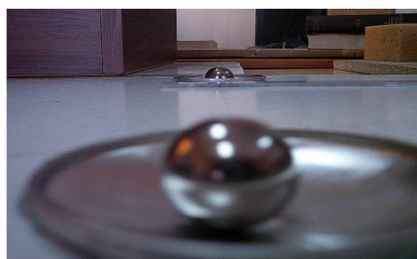
Figure 3.2. Reduced scale model of the rolling pendulum isolation system
