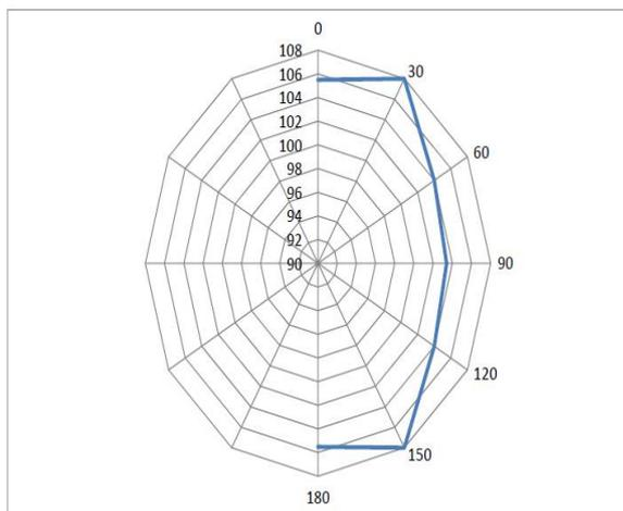
Fig.6. The angular diagram of air-jet stem generator with reflector disk: resonator distances  $\Delta=1.2$  mm and supply pressure  $p = 0.1$  MPa.
