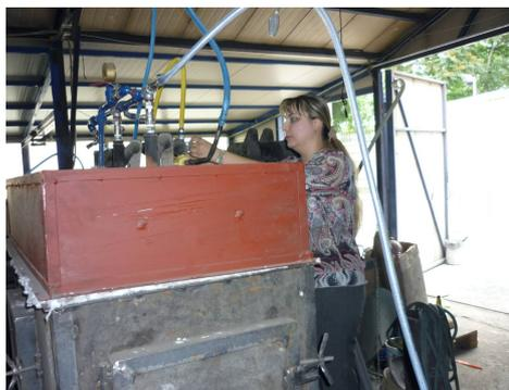
Figure 2. Testing the furnace with 3 smaller gas burners.
