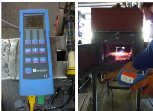
Figure 4. Combustion gas analyzer MINILYZER 02.
