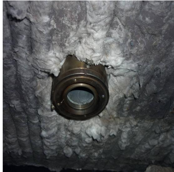
Figure 3. The inside of the oven (the sonic generator is located in the ceiling of the oven).
