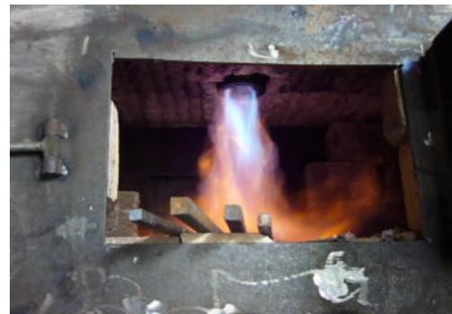
Figure 9. The operation of the burner with the sonic generator to supply air pressure of 0,15 MPa, the slot generator of 0,25 mm.
