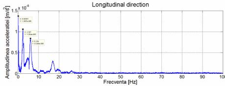
b) Superstructure longitudinal direction of movement
