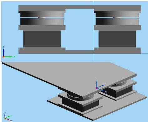
Fig. 2. Three-dimensional assembly model for a hybrid isolation system
