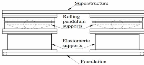
Fig. 1. Schematic representation for the hybrid isolation system model assembly
