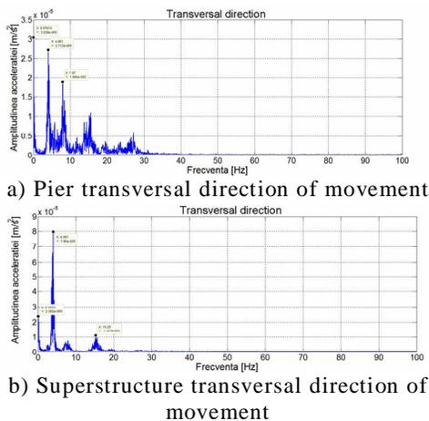
Fig. 4. Experimental values obtained for testing rolling pendulum system in transversal direction
