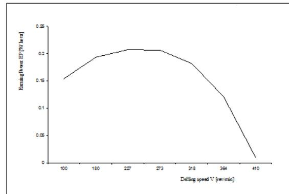
Fig. 4 The variation of the Earning Power depending on drilling speed
