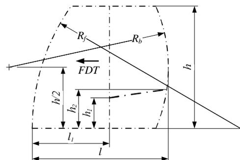
Fig. 4 – The profile of a cabin with curve overall geometry (both front side and back side of the cabin are curved)
