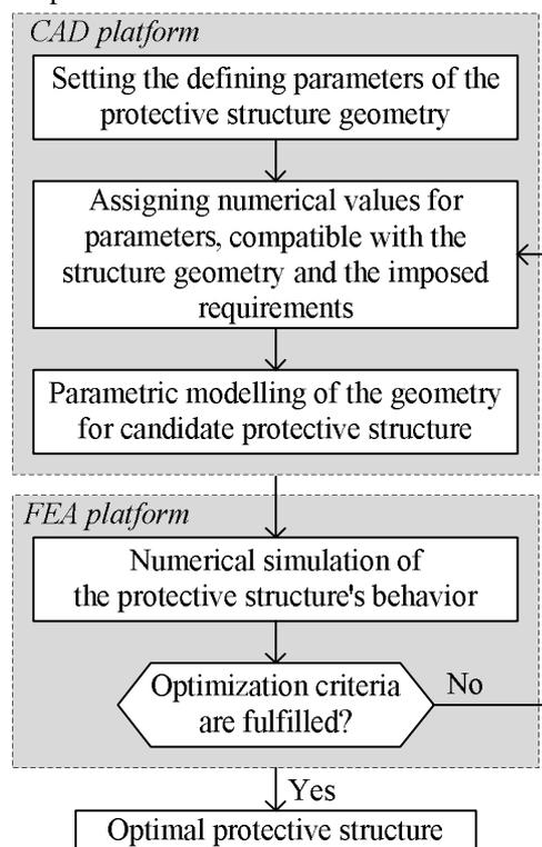
Fig. 1 – Optimization algorithm of the protective structures
