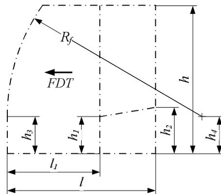
Fig. 3 – The profile of a cabin with curve overall geometry (only the front of the cabin is curved)
