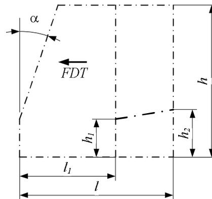
Fig. 2 – The profile of a cabin with polyhedral overall geometry
