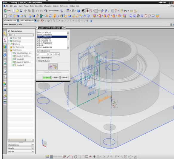
Fig. 2 Sketch used for command "Revolve"
