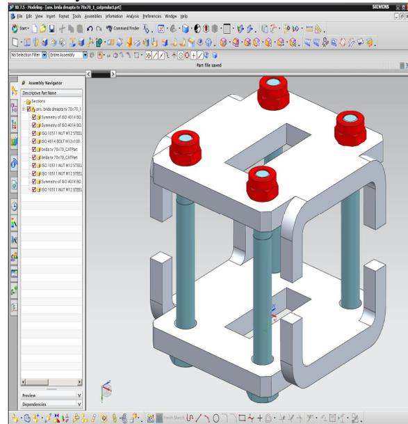
Fig. 4 The coupling flange subassembly.
