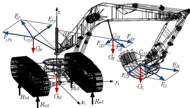
Fig.7. Forces that occur in the centers of mass of the excavator during rotation
