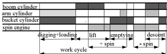
Fig. 1. The operating cycle of an excavator
