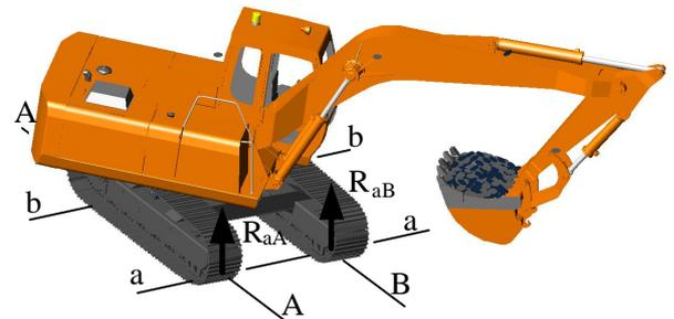
Fig. 2. Lines of overturning
