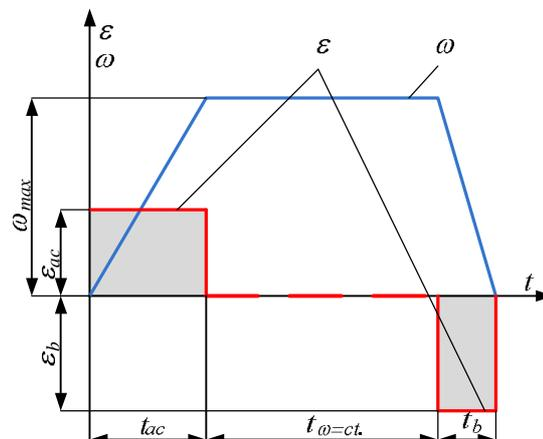
Fig. 4 Diagram angular velocities and accelerations
