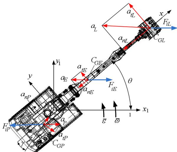
Fig. 6. The accelerations of mass centers of components
