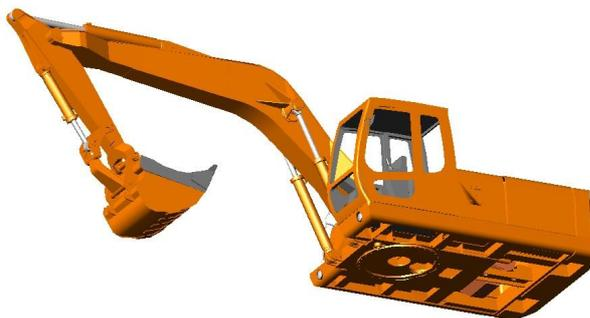
Fig. 3. Rotating Platform and working equipment
