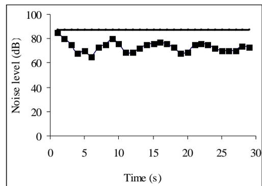
Fig. 6 The sound level on the navigation bridge while the ship starts from the shore (—)87dB, limit value [8]
