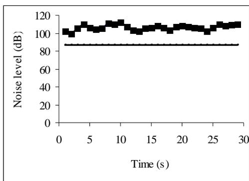
Fig. 10 Sound level inside the engines room (idling with generator engine);
