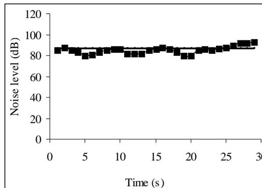
Fig. 9 The sound level on the main deck while the ship performs the mooring manoeuvre
