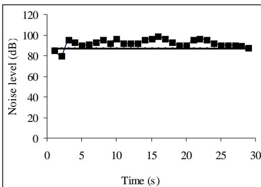
Fig. 8 The sound level on the main deck while the ship is running
