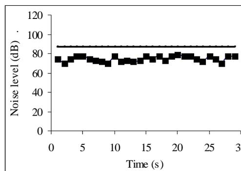
Fig. 11 Sound level in the command cabin while the ship is idling with generator engine generator;
