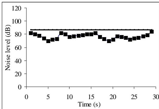
Fig. 12 Sound level inside the rest area while the ship is running;
