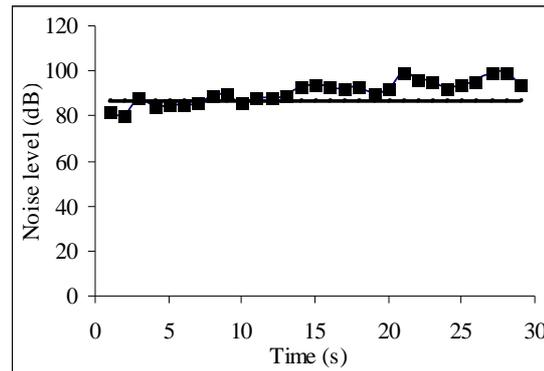
Fig. 13 Sound level inside the rest area while the ship performs the mooring manoeuvre;
