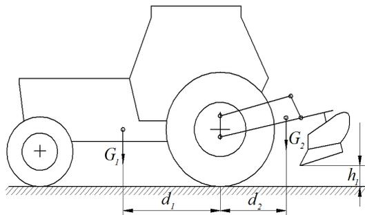
Figure 2.1 Schematic representation for tractor with ploughing equipment mounted [7]
