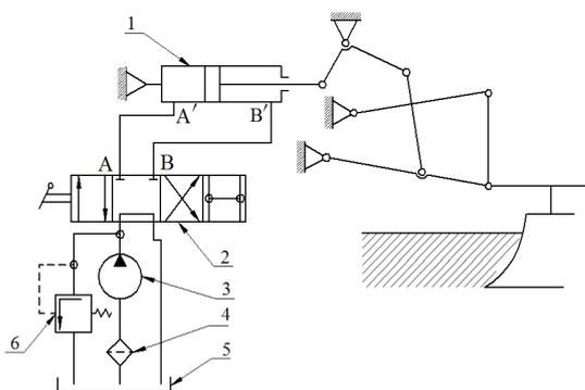
Figure 3.2. Hydraulic components diagram for suspension mechanism [11]
