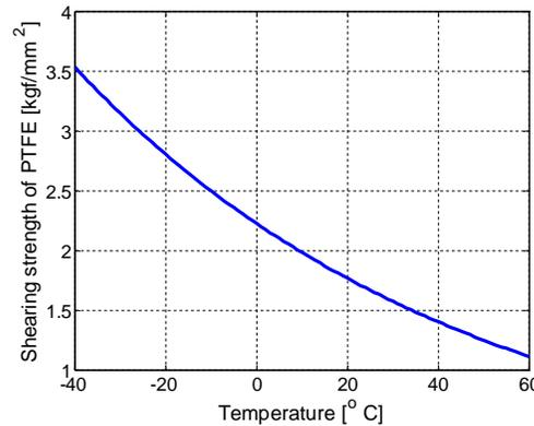
Fig. 3 Dependence of the shearing strength on temperatures
