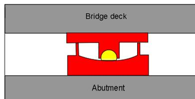
Fig. 1 Friction pendulum sliders
