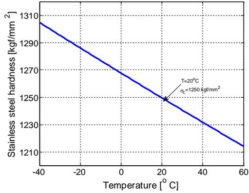
Fig. 2 The allure of hardness steel versus temperature
