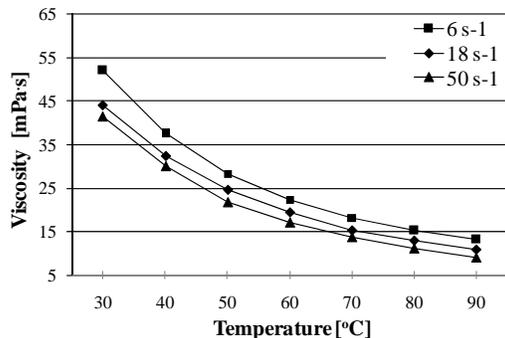
Fig. 2. Dynamic viscosity / temperature variation
