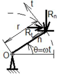
Fig. 3. Schematic representation of the forces that act on the palette
