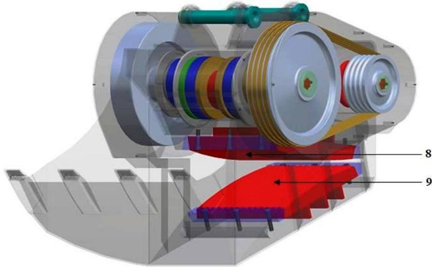
Fig. 2 The 3D model presentation of the equipment type cup crushed
