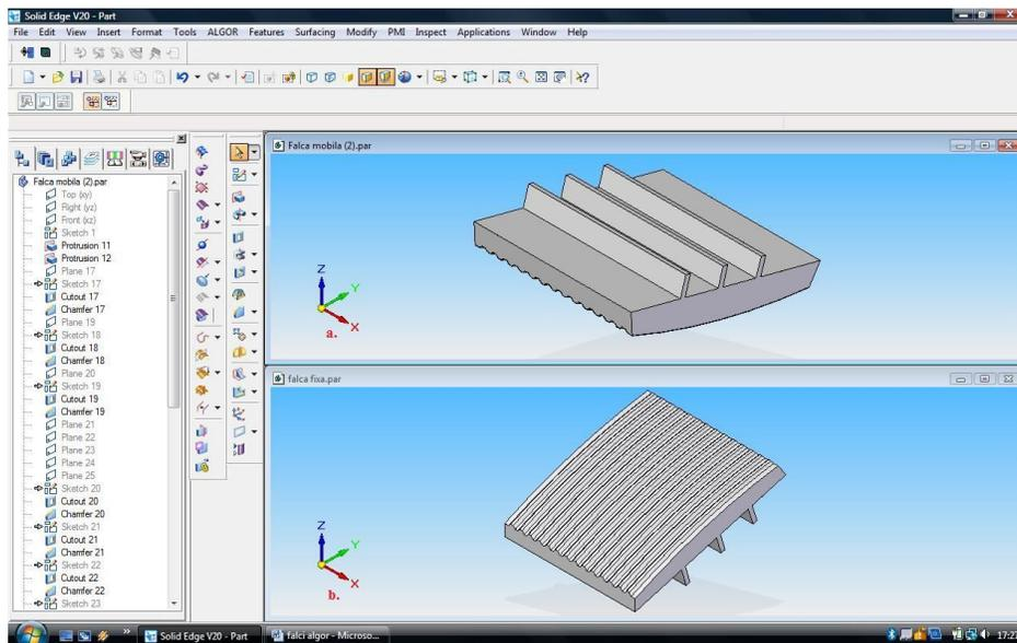
Fig. 3 Solid model of armor: a) mobile armor, b) fixed armor
