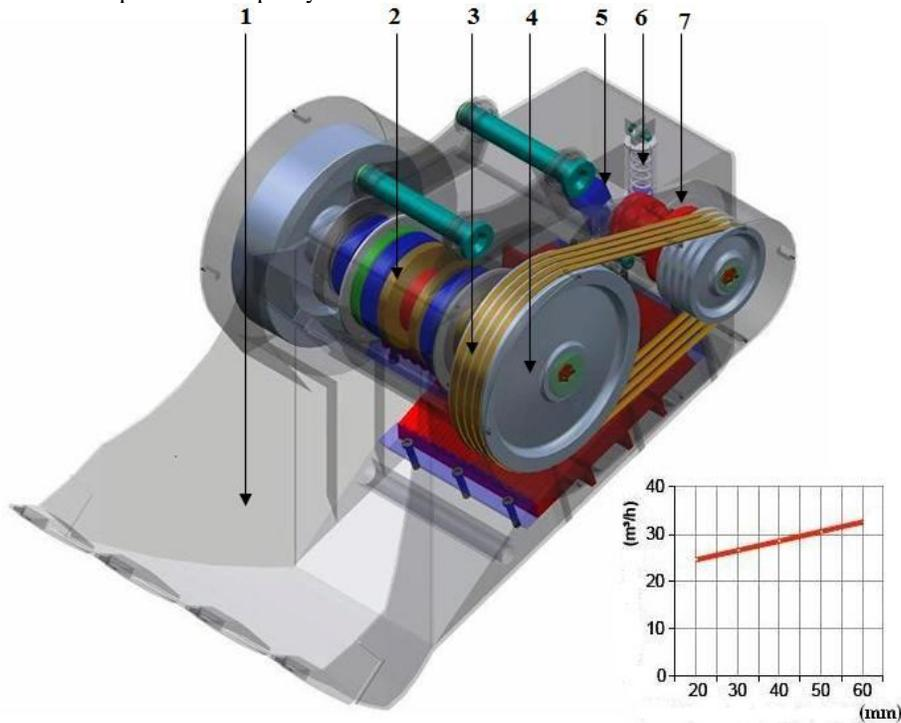
Fig.1a The 3D model presentation of the equipment type cup crushed m<sup>3</sup>/h
