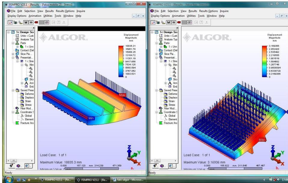
Fig. 4 The result of the analysis of movement: a) mobile armor, b) fixed armor
