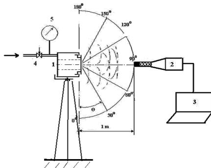
Fig. 6. Pattern of performing measurements at different angles of the generator's acoustic emission: 1 - radial generator, 2 - sound meter, 3 - laptop,  $\theta$  - measurement angle
