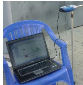
Fig. 3. Sonometer Solo 0.1 dB with laptop during measurements
