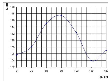
Fig. 7. The level of acoustic intensity  $L$  depending on the angle of emission  $\theta$  of the gasodynamic radial generator (working pressure  $p = 0.20$  MPa, slot nozzle  $\delta = 0.50$  mm)
