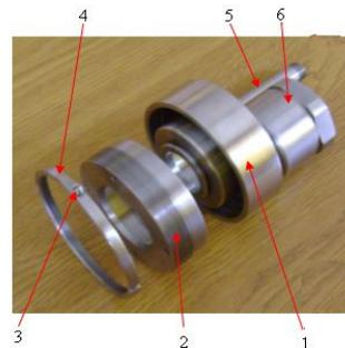
Figure 2. Photo experimental gasodynamic radial sonic generator: Photo of the overall radial type generator gazodinamic: 1 - resonator; 2 - radial nozzle, 3 - pin fastening, 4 - nozzle retaining nut, 5 - air supply pipe work
