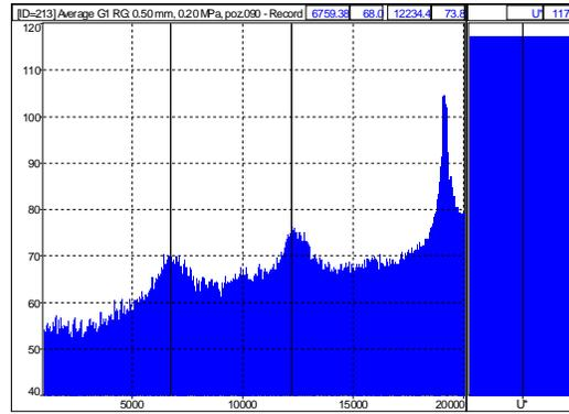
Fig. 5. Pulsation spectrum at working pressure  $p = 0.20$  MPa,  $\delta = 0.50$  mm, the angle of emission  $\theta = 90^\circ$ .
