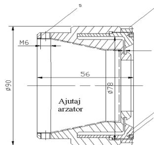
Figure 1. Experimental gasodynamic radial sonic generator: 1 - resonator, 2 - nozzle, 3 - nut, 4 - connection hose; 5 - air supply pipe work
