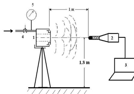
Fig. 4. Acoustic performance measurement scheme:
