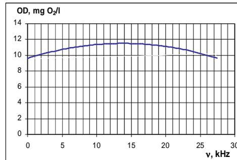
Figure 8. The variation of dissolved oxygen with the ultrasound frequency
