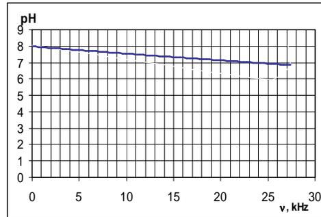
Figure 5. The variation of pH with the ultrasound frequency
