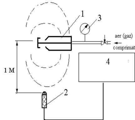
Figure 4. The acoustic testing diagram: 1- sonic generator, 2-microphone, 3-manometer, 4- testing system „Brüel & Kjør”
