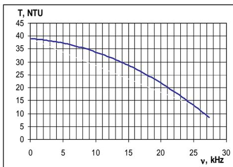
Figure 6. The variation of turbidity with the ultrasound frequency
