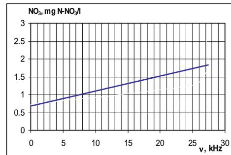
Figure 9. The variation of nitrate content with the ultrasound frequency
