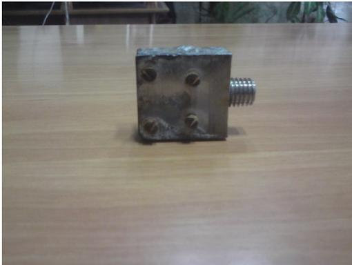
Figure 3. The air-jet sonic generator with two resonators
