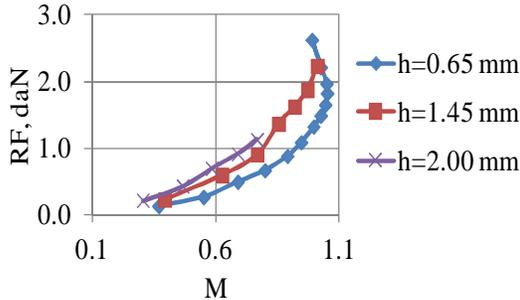
Fig. 10. Reaction force (daN) in function of jet velocity and slot size (*h*) of radial nozzle at its diameter ratio  $D_a/D = 0.25$  (transonic regime)
