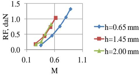
Fig. 9. Reaction force (daN) in function of jet velocity and slot size (*h*) of radial nozzle at its diameter ratio  $D_a/D = 0.32$  (subsonic and transonic regimes)
