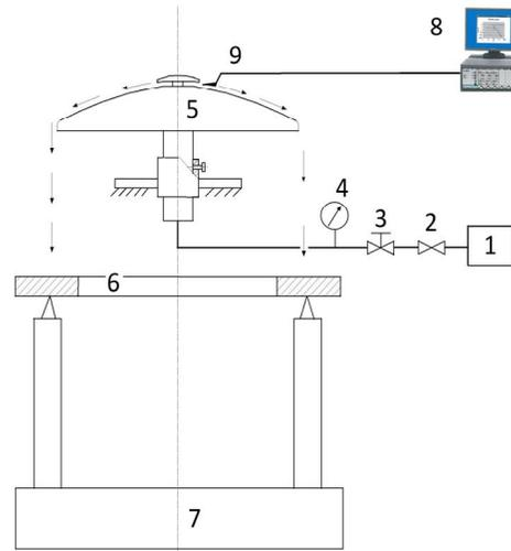
Fig. 3. Test rig for reaction force measurements: 1 – compressor; 2 – valve; 3 – expansion valve; 4 – manometer; 5 – Coanda nozzle; 6 – ring; 7 – aerodynamic balance; 8 - Streamline Pro Anemometer System; 9 - conical film probe 55R42
