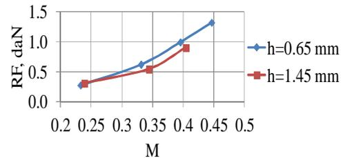
Fig. 6. Reaction force (daN) in function of jet velocity and slot size ( $h$ ) of radial nozzle at its diameter ratio  $D_a/D = 0.61$  (subsonic regime)
