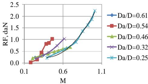
Fig. 11. Reaction force (daN) in function of Mach number and diameter ratios at slot size  $h = 1.45$  mm
