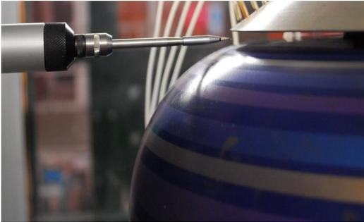
Fig. 5. Probe 55R42 during the velocity measurements
