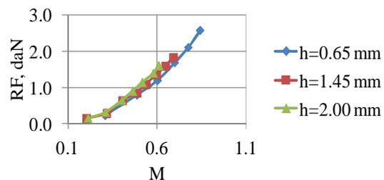
Fig. 8. Reaction force (daN) in function of jet velocity and slot size ( $h$ ) of radial nozzle at its diameter ratio  $D_a/D = 0.46$  (subsonic regime)
