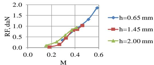
Fig. 7. Reaction force (daN) in function of jet velocity and slot size ( $h$ ) of radial nozzle at its diameter ratio  $D_a/D = 0.54$  (subsonic regime)
