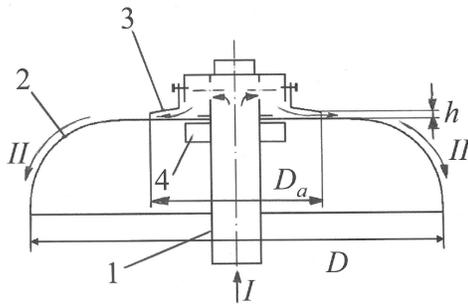
Fig. 1. Coanda nozzle: 1-air supply pipe; 2- Coanda airfoil; 3-radial nozzle; 4-binding nut; I-compressed air; II-radial jet; D – Coanda airfoil diameter;  $D_a$  – radial nozzle diameter; h – slot size
