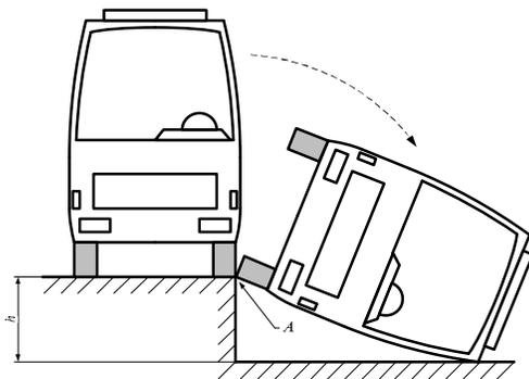
Fig. 2 – Experimental test of lateral rollover, according to ECE R66
