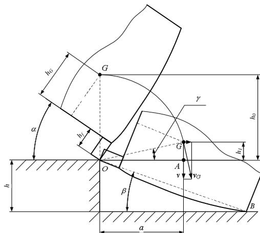
Fig. 3 – The calculus scheme of the translational speed at the time of impact
