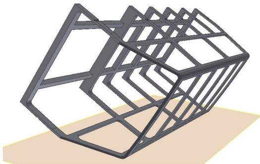
Fig. 3 – Overturned geometric model of the bus structure
