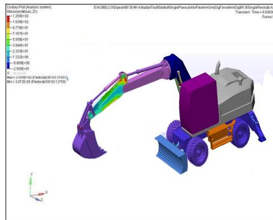
Fig. 7. Modeling arm no.1 after meshing
