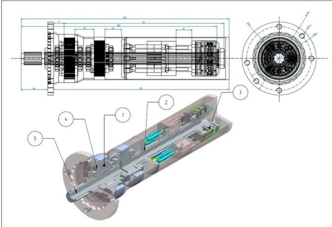
Fig.3 The 3D modeling of the hydro motor subassembly
