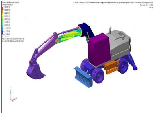
Fig. 8. Modeling arm no.2 after meshing
