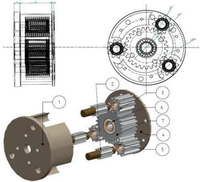
Fig.5. Subassembly of planetary gear
