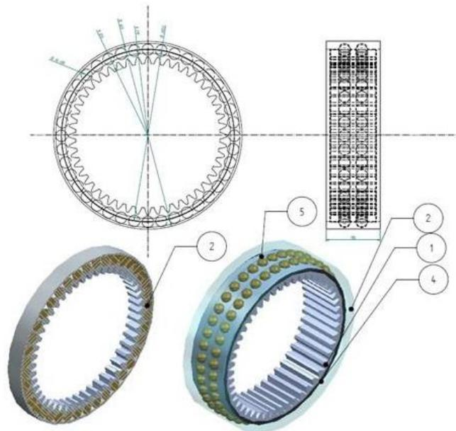
Fig.4. Subassembly of special radial-axial bearing
