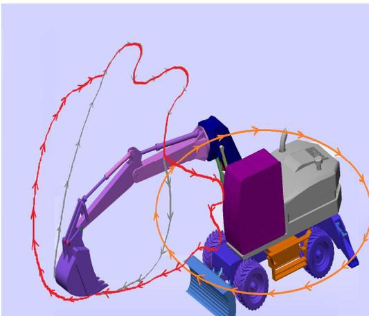
Fig. 10. Access areas of the excavator bucket
