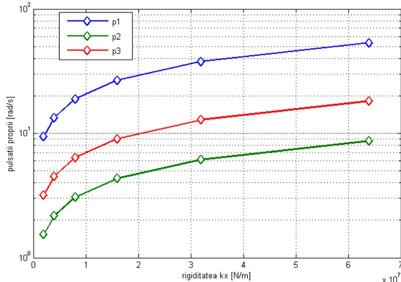
Fig. 2. The dependence between the natural pulsations of the system and the rigidity in the horizontal direction
