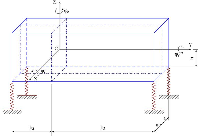
Fig.1. Model of the rigid system with six degrees of freedom, elastic supported in four points on inferior base, with a longitudinal vertical plane of symmetry
