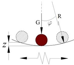
Figure 1. Description of rolling pendulum motion concept
