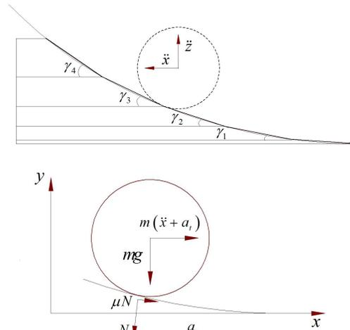
Figure 2. Schematic representation of planar model view for rolling spherical part
