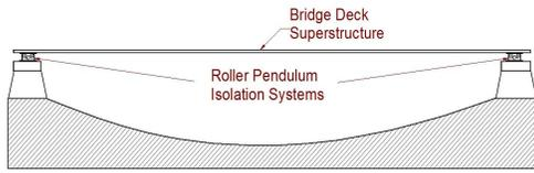
a) 2D - model view of a bridge superstructure isolated with RPS
