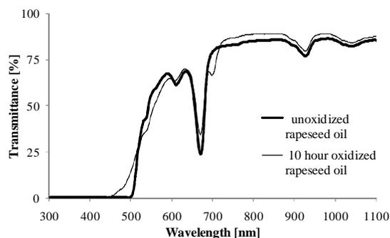
Fig. 5. Rapeseed oil transmittances oxidized for 10 hours at a temperature of 130°C
