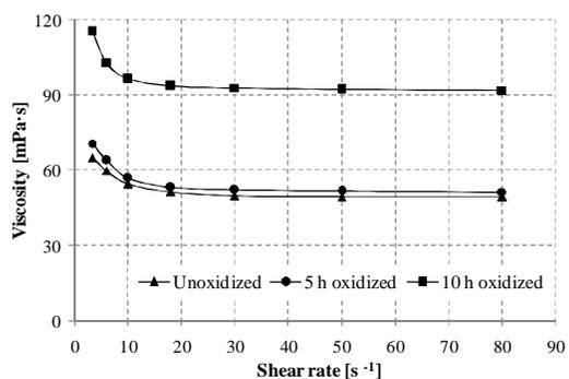
Fig 7. Variation of viscosity with shear rate for oxidized rapeseed oil at 130°C
