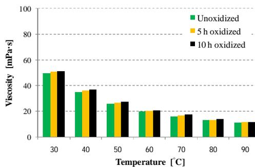
Fig. 8. Variation of viscosity with temperature for oxidized rapeseed oil at the temperature of 120°C
