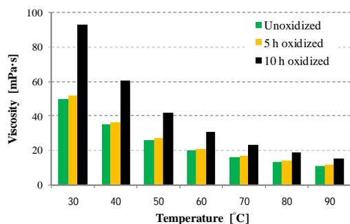
Fig. 9. Variation of viscosity with temperature for oxidized rapeseed oil at the temperature of 130°C
