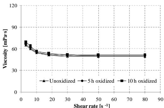
Fig.6. Variation of viscosity with shear rate for oxidized rapeseed oil at 120°C
