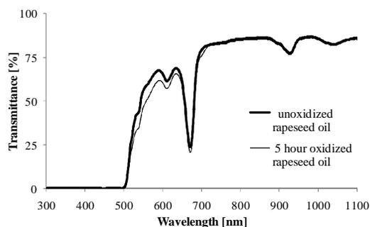
Fig. 4. Rapeseed oil transmittances oxidized for 5 hours at a temperature of 130°C
