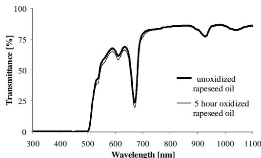
Fig. 2. Rapeseed oil transmittances oxidized for 5 hours at a temperature of 110°C
