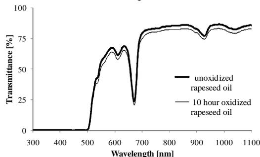
Fig. 3. Rapeseed oil transmittances oxidized for 10 hours at a temperature of 110°C
