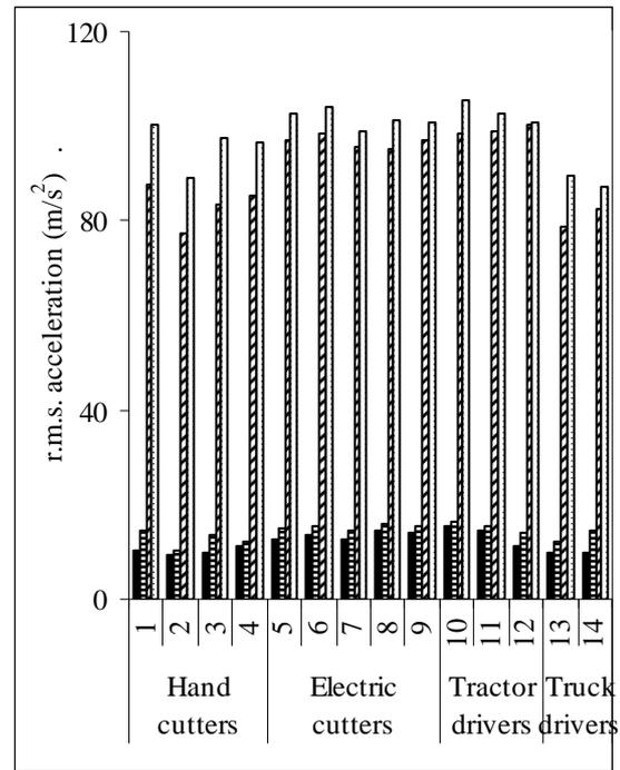
Fig. 2 Mean magnitude of root mean square of the frequency weighted and unweighted acceleration: (■) weighted (Dominant axis); (≡) weighted (Vector sum); (//) unweighted (Dominant axis); (⊙) unweighted (Vector sum)
