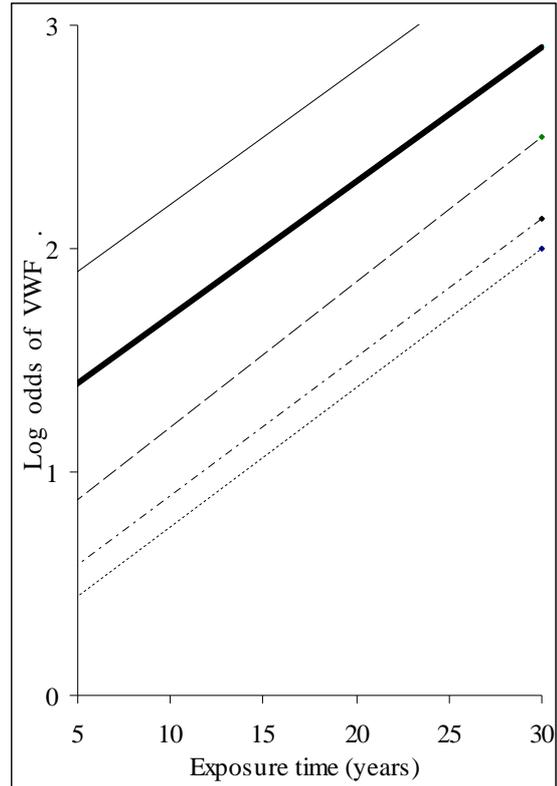
Fig. 4 Log odds of occurrence of vibration induced white finger according to the 8h frequency weighted energy equivalent acceleration and duration of vibration exposure (—):  $A(8) - 1m/s^2$ ; (—):  $A(8) - 2.5m/s^2$ ; (---):  $A(8) - 5m/s^2$ ; (- · -):  $A(8) - 10m/s^2$ ; (- - -):  $A(8) - 15m/s^2$ ;
